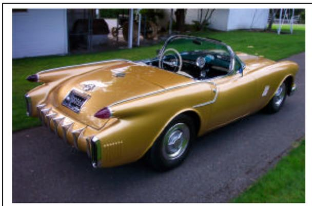
This two-seat 1954 Oldsmobile F-88 with Corvette sized fiberglass-body has a hopped-up 324cid Olds V8 engine producing 250 horsepower and a 4-speed Hydra-Matic transmission.
